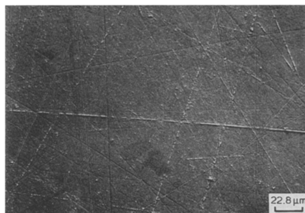
Fig. 5. SEM photomicrograph showing the mechanism of the levelling action of TBACl at the beginning of Zn electrodeposition. I = -0.3\text{ mA} , t = 30\text{ s} . 0.5\text{ M ZnCl}_2 + 1\text{ M NaCl} + 40\text{ mg l}^{-1} TBACl.
